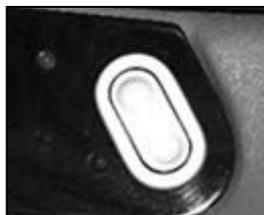
Unique Aluminium window switches to match the other switches and controls. Fits Griffith 500 and Chimaera. Also fits Griffith 4.0/4.3 window switches and heater controls. (2 pairs required).
