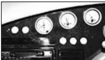
Replacement solid aluminium caps designed specifically to match the style of the instruments.
