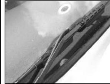
Replaces the loop pipe with a blade mounted 3 jet head system. The wiper blade incorporates 3 individual jets. The whole unit which is easy and quick to fit provides a great improvement to the existing version.
