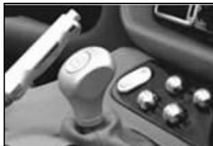
Cobra shaped and specifically designed specifically for TVRs. Machined from solid aluminium and anodised for durability.
